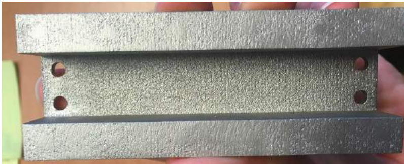
Figure 5.2 – Picture of the bottom surface of the bladed rail prototype. The high roughness of the surface is visible at naked eye.
