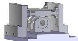
*Figure 1:* 1 *d.o.f* mockup with roller guiding.
