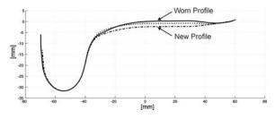
Fig. 2. Contact points between a new rail profile and (a) new wheel profile; (b) a worn wheel profile.
