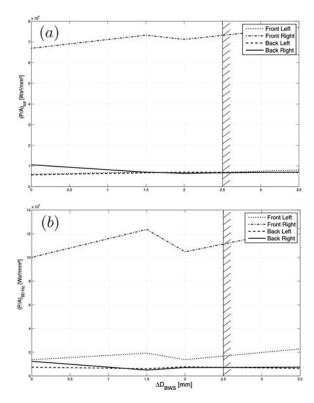
Fig. 10. Energy dissipated in contacts of the front bogie as a function of an increasing diameter difference of the back wheel set (a) in the whole frequency range; (b) between 53 Hz and 67 Hz.
