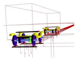
Fig. 18. Multi-body model of the vehicle-track system.
