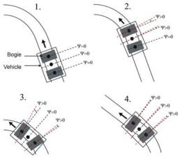
Fig. 4. Four stages of a bogie passing a curve.
