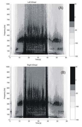
Fig. 5. STFT of the frictional power dissipated in the (a) left and (b) right wheel-rail contact of the back wheel set of the front bogie.
