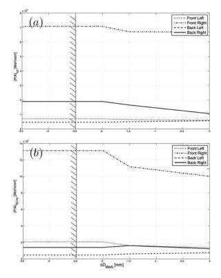
Fig. 9. Energy dissipated in contacts of the front bogie as a function of an decreasing diameter difference of the back wheel set (a) in the whole frequency range; (b) between 53 Hz and 67 Hz.
