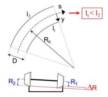
Fig. 3. Simplified drawing of a curved track; Lateral position of the wheel set on the track.
