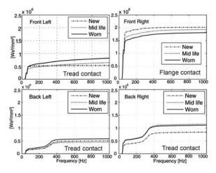
Fig. 6. RMS values of the frictional power dissipated in wheel-rail contacts of the front bogie for new, intermediate and worn profiles.
