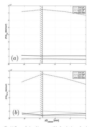
Fig. 14. Energy dissipated in contacts of the front bogie as a function of an increasing diameter difference of the back wheel set (a) in the whole frequency range; (b) between 53 Hz and 67 Hz
