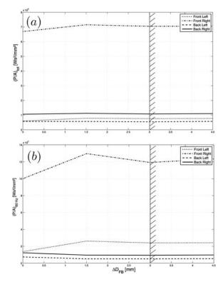
Fig. 12. Energy dissipated in contacts of the front bogie as a function of an increasing bogie wheels diameter difference (a) in the whole frequency range; (b) between 53 Hz and 67 Hz.
