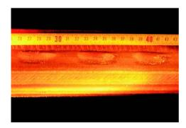
Fig. 17. Picture of a corrugated rail.
