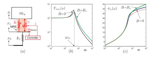
**Figure 1.** (a) Model of MRE isolator; (b) Transmissibility  $T_{x_0x_s}(\omega)$  and (c) RMS value  $\sigma_{x_s}(\omega)$  of a MRE isolator for two values of B: B = 0 (blue curve) and  $B = B_s$  (green curve).
