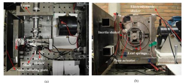
Figure 1 The experimental test bed and inertia shaker
