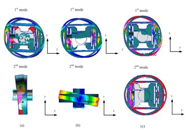
**Figure 3** The first two mode shapes of the inertia shaker for a piezo element with Young's modulus of 76.5 GPa (left), 5 GPa (middle) and 0.3 GPa (right).
