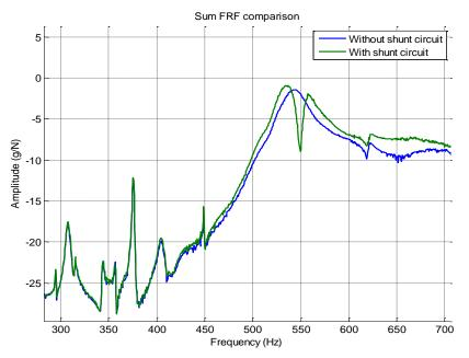
Figure 9 A Comparison of Sum- FRFs with and without shunt circuit
