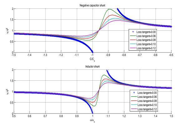
Figure 2 The effective Young's modulus of piezo element connected to a negative capacitor or an inductor, for a range of loss values and for various values of the capacitance and excitation frequency.
