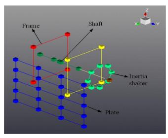
Figure 4 Schematic representation of the measurement setup, with indications of the accelerometers attached to the structure at various components.
