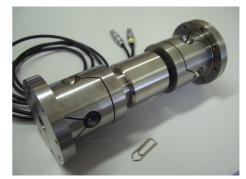
Figure 1: Actuator with two prototype hinges.
