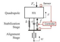
Figure 1: Model of a stabilized system with a single d.o.f.
