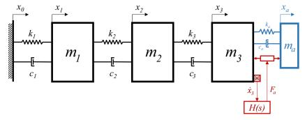
**Fig. 1.** Simplified model of a flexible structure with an AMD/HMD. (Blue: passive part, red: active part). (For interpretation of the references to color in this figure caption, the reader is referred to the web version of this paper.)
