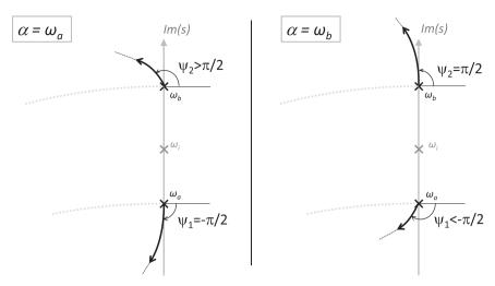
**Fig. 4.** Departure angles on the root locus, left:  $\alpha = \omega_a$ , right:  $\alpha = \omega_b$ , without structural damping.
