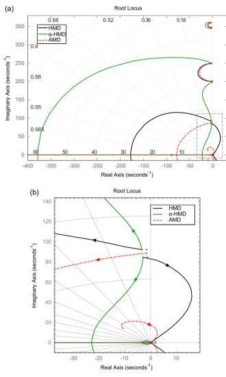
**Fig. 2.** (a) Root locus for AMD, HMD and  $\alpha$ -HMD. (b) Detail near the origin of the root locus. (For interpretation of the references to color in this figure caption, the reader is referred to the web version of this paper.)
