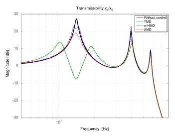
**Fig. 5.** Transmissibility function  $x_3/x_0$  for various control devices.
