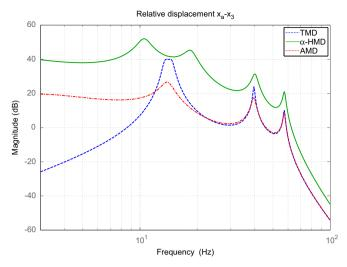
**Fig. 6.** Relative displacement spectrum of the actuator  $(x_a - x_3)$  for a broadband ground disturbance  $(x_0)$ .
