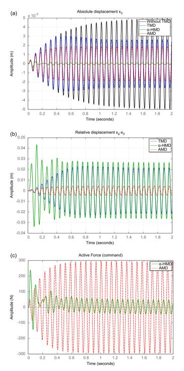
**Fig. 8.** Time response to a ground disturbance:  $\ddot{x}_0 = A \sin(\omega_1 t)$ : (a) absolute displacement  $x_3$ ; (b)Relative displacement of the actuator ( $x_a - x_3$ ). (c) Active force of the actuator (command).
