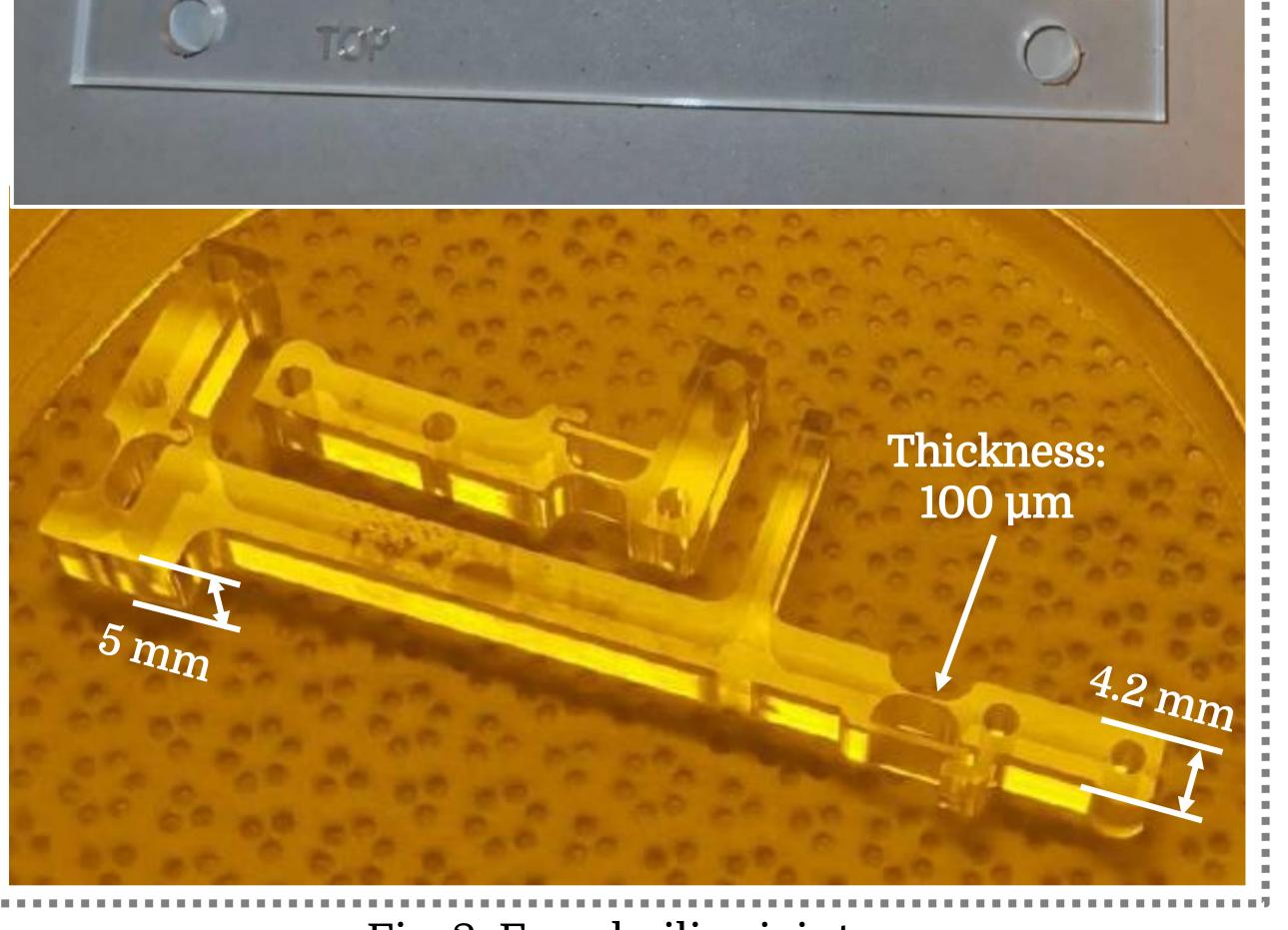
Fig. 3: Fused-silica joints.
