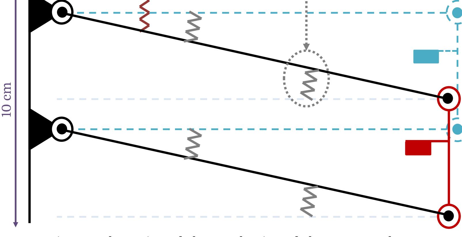
Fig. 2: Schematics of the mechanics of the sensor. The "four-bars" mechanism guarantee the translation motion of the mirror.
