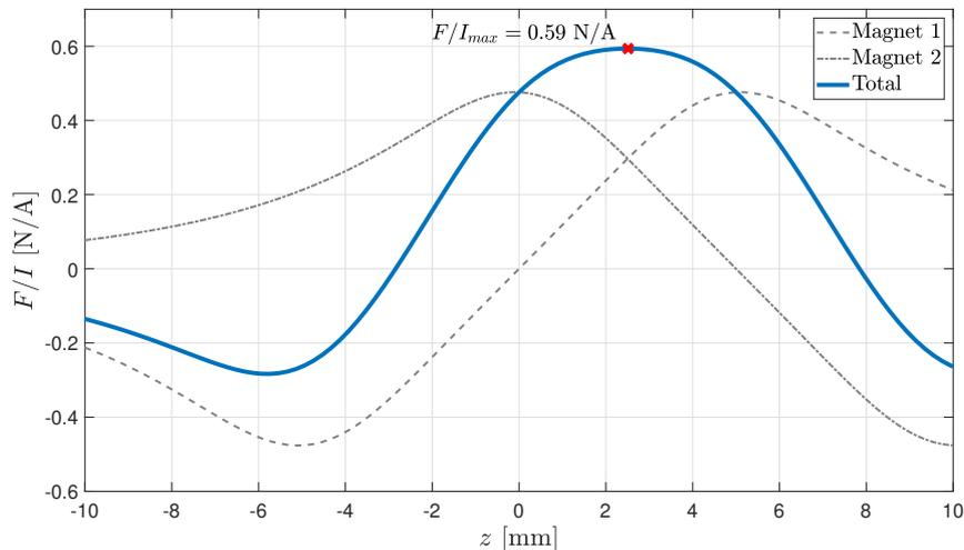
Figure 5: Force per unit current of the custom voice-coil.  $z$  represents the distance of the magnet assembly to the coil center. The Lorentz forces applied on each individual magnets are shown as grey lines, and the resulting force is shown in blue. The voice-coil has a maximum force constant of 0.6 N/A in the optimal position.
