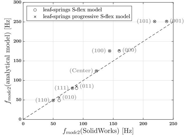
Figure 12: Comparison between the torsion mode results of the numerical approach and the analytical approach
