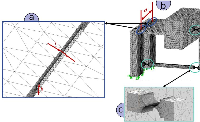
Figure 10: The simplistic design used for the modal analysis (b). The mesh control used for the flexure hinges is 0.1 mm (a and c). The input parameters of the experiment are  $d$ , the distance between the centers of the leaf-springs,  $h$ , their thickness and  $l$ , their length.
