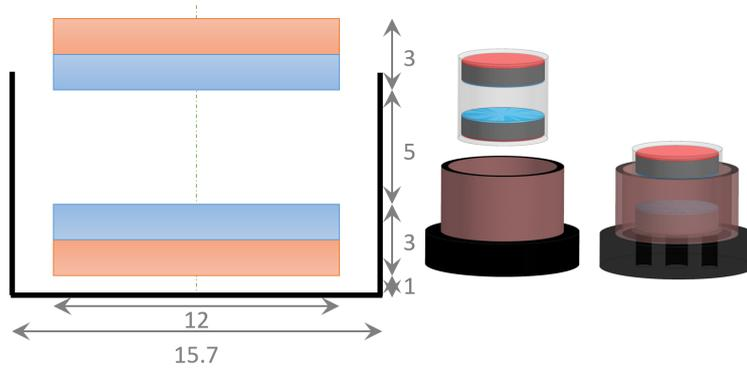
Figure 4: Schematic drawing of the double magnet voice-coil (left) and CAD view (right). The Neodymium magnets are shown as the blue/orange blocks, the coil is drawn in black and characteristic dimensions are shown in grey. The double magnet assembly is embedded in a casing made of a non-magnetic material.
