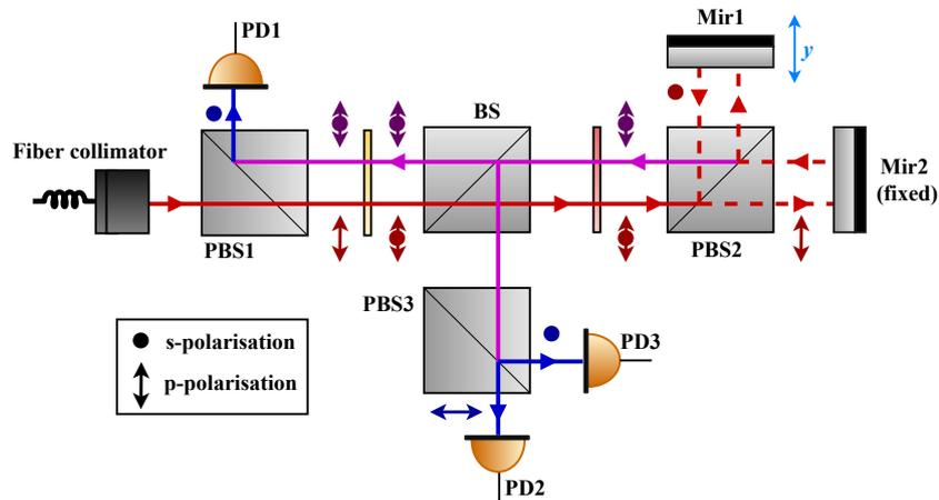
Figure 3: Quadrature interferometer optical scheme. The optical path to the retro-reflecting mirrors Mir1 and Mir2 is shown in red, while the reflected path is shown in purple. The light intensities detected at the photodiodes are shown in blue. The polarisation state of the laser beam is indicated using arrows (p-polarisation) or a dot (s-polarisation) [16].
