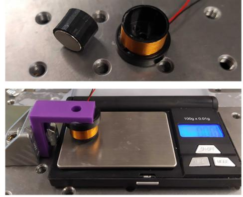
Figure 6: Force output of the custom voice-coil actuator fed with DC current (left) and experimental setup (right). The voice-coil was mounted on a scale and fed with DC current. The weight reading on the scale can be upconverted to a force reading measurement. The force constant of 0.6465 N/A have been measured.
