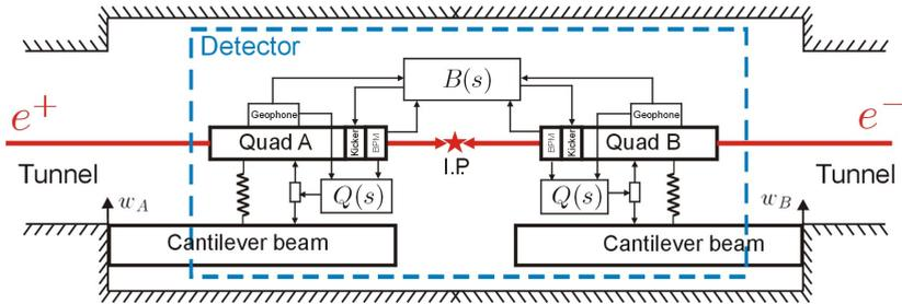
Figure 2: Simplified layout of the final focus of a linear particle collider.
