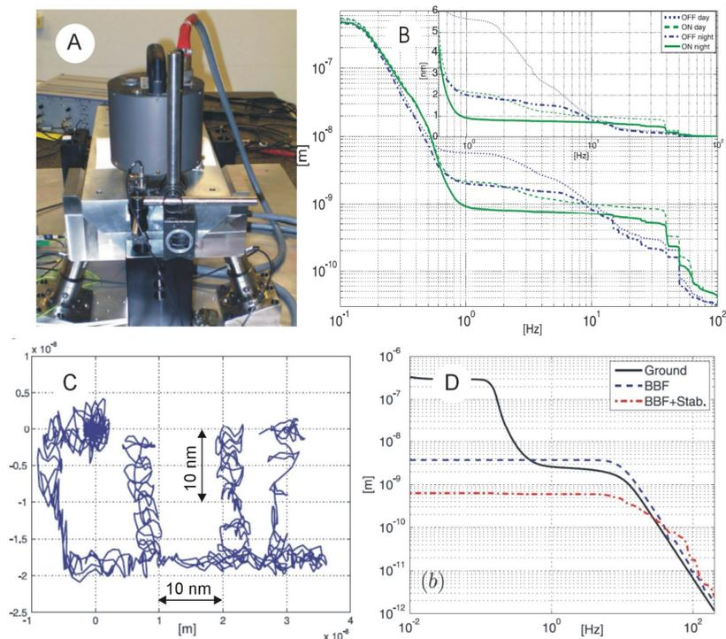
Figure 4: (a) Test bench; (b) Transmissibility between the motion of the ground and the quadrupole; (c) Illustration of the nano-positioning capability; Integrated RMS of the ground, the beam jitter with B(s), the beam jitter B(s) and Q(s).
