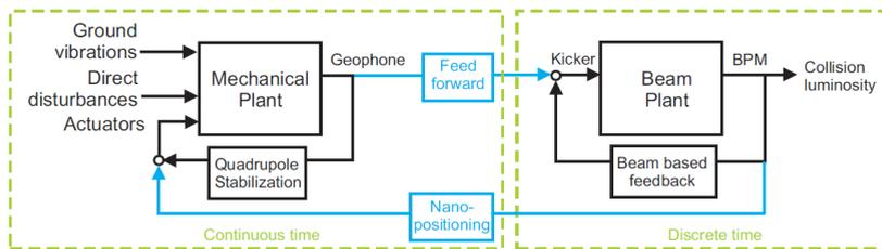
Figure 3: Block diagram of the final focus of a linear particle collider.
