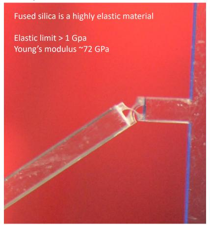
Thanks to the high aspect ratio of the manufacturing process, we are able to produce monolithic compliant mechanisms
