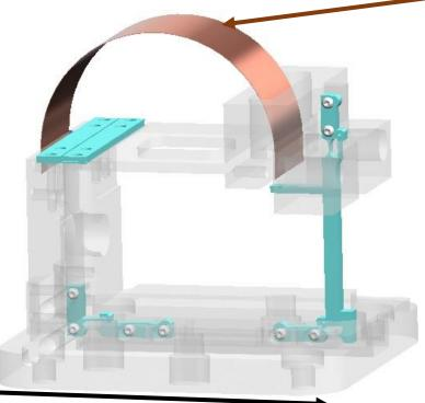
Glass can be used for compliant joints to reduce drift and thermal noise (depending on the stress ratio between the joint and the suspension)
