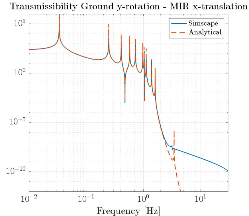
Analytical model provides the correct shape after 2 Hz
